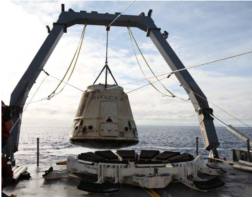
Figure 2-17. Recovery A-frame Crane Operation
