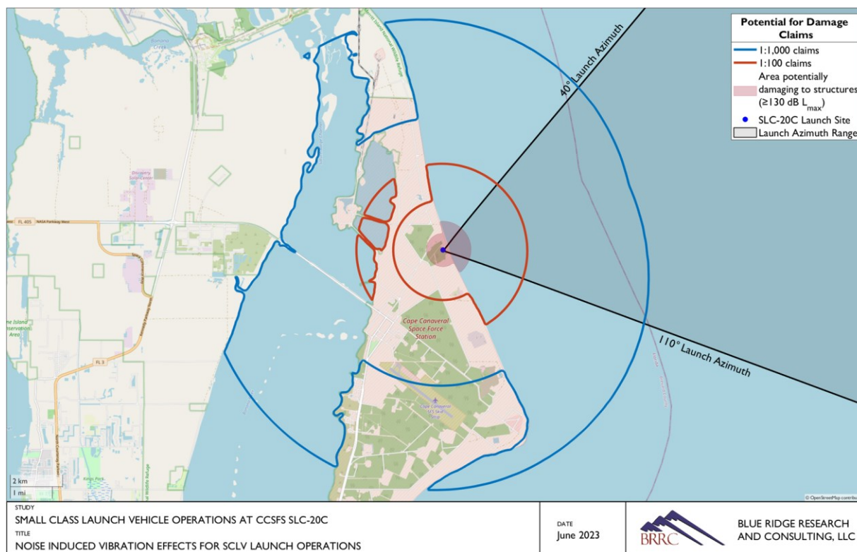
Figure 12. Potential for damage claims contours for SCLV launch operations over the azimuth range (40° - 110°).
